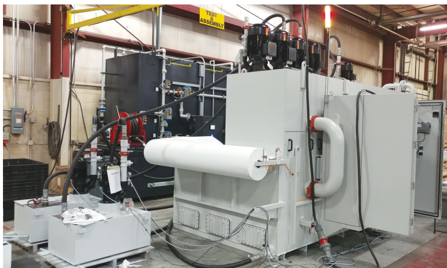
Hoffmann Filter UBF 300 undergoing operational testing prior to shipment.
